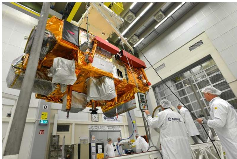
***Payload module of MetOp-C is being prepared for transport.***
